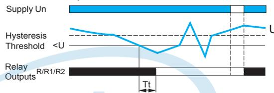
Tt: time delay after crossing of threshold
