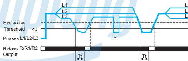
$T_t$ : time delay after crossing of threshold
