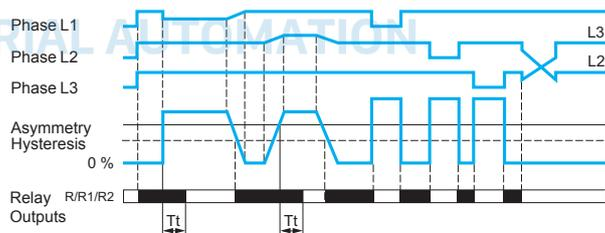
Tt: time delay after crossing of threshold (adjustable on front panel)
