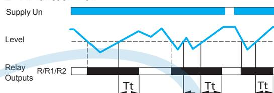
Tt: time delay after crossing of threshold
