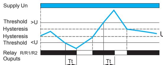
Tt: time delay after crossing of threshold
