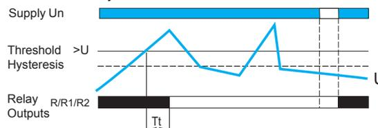
Tt: time delay after crossing of threshold
