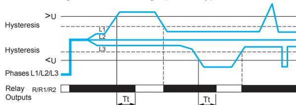
$T_t$ : time delay after crossing of threshold (adjustable on front panel)
