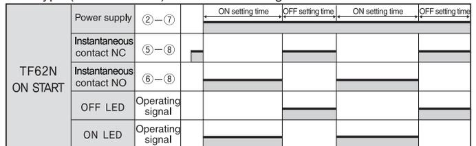
■ F type (Time - limit 2c) - Same ON setup time will be applied to the output A and B
