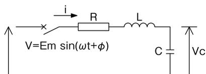
Fig. 3-26 Capacitor residual voltage
