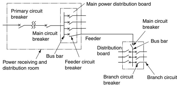
**Fig. 3-3 Wiring and load protection using MCCBs (Overload and intermediate overcurrent region)**
