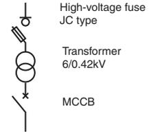
**Table 3-7 (a) Selective trip coordination between MCCB and 6kV power fuse**
