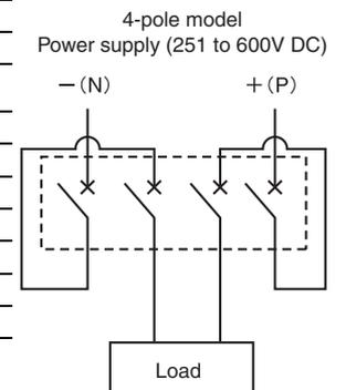
Notes: • The instantaneous DC tripping current for AC/DC models is approximately 140% max. of the AC rating. Models with the same instantaneous tripping current as the operating characteristics curve given in a catalog or other documentation can be produced if "C5" or "C6" is specified at the end of the model number. (DC-only models)
