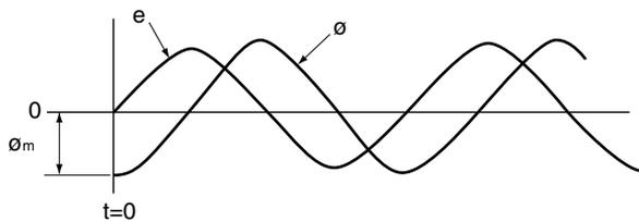
Accordingly, assuming that excitation of the transformer is started at  $t=0$ , the magnetic flux  $\phi$  must be 0 if the prior residual flux is 0. The flux exhibits  $\phi$  as shown in Fig. 3-20, which is far above the core saturation flux  $\phi_s$  of the transformer. However, as the magnetic flux  $\phi$  is saturated to the value of  $\phi_s$  for the
