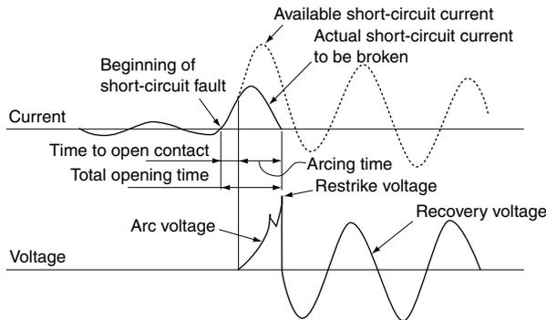
When a short-circuit fault occurs and a short-circuit current flows, the instantaneous trip device is actuated to quickly open the contacts. An arc is generated between the contacts the moment the moving contact separates from the stationary contact.
