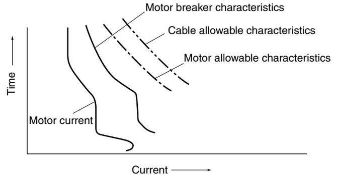
Fig. 3-17 Protective structure for motor circuits
