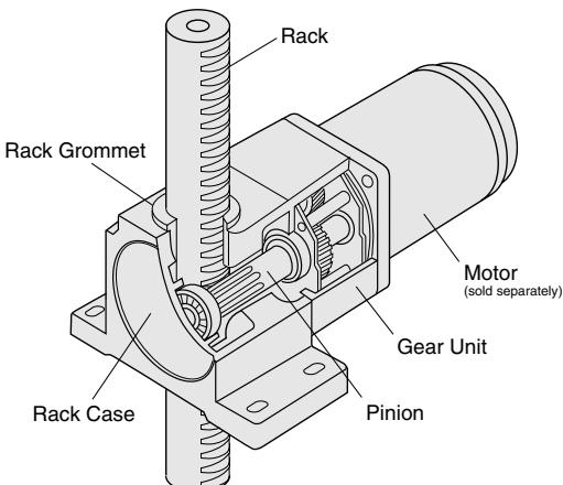
The direction of rack movement is determined by the direction of motor rotation.
