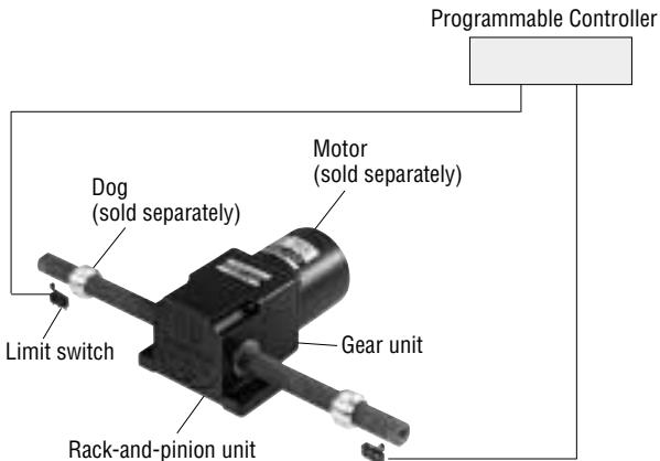
The linear heads come with a rack-and-pinion unit and a reduction gear unit. Motors and dogs are sold separately. Linear heads may be combined with any standard AC motors. Any limit switches available on the market can be used. Three rack speeds are available for a given frame size, by changing on the speed reduction ratio. The rack movement is controlled using a brake pack, programmable controller or relays.
