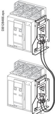
Complete assembly with 2 adaptation fixtures + cables
