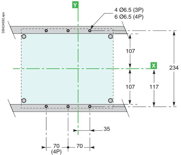
**Note:** Mounting parameters for electrically operated devices are identical to those for manually operated devices.
