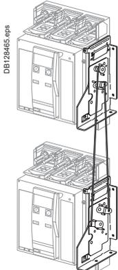
Complete assembly with 2 adaptation fixtures + rods
