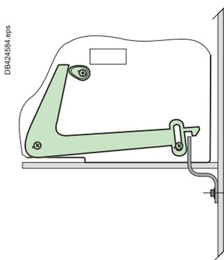
**Note:** The door interlock may be mounted on either the left or right-hand side of the chassis.
