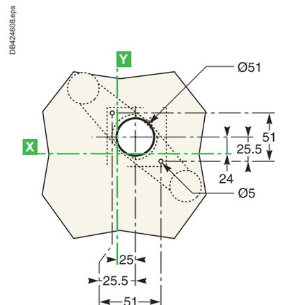
Note: X and Y are the symmetry planes for a 3-pole device.
