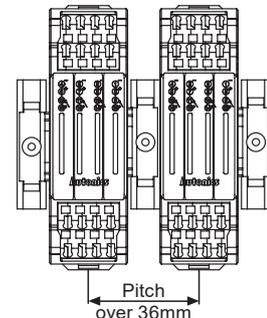
※Pitch is interval between SSRs.
