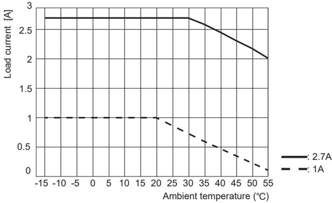
When installing ASL-L01, load current by ambient temperature for SSRs interval
