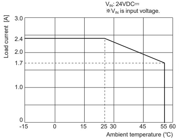
When installing ASL-L04 individually, load current by ambient temperature for SSRs interval
