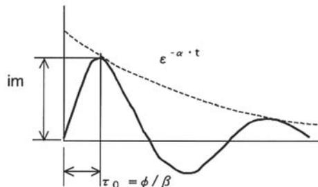
Since the natural frequency at this time is as follows:  $f = \omega/2\pi$ , equation (1) yields  $\omega = \beta$ , and so
