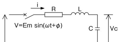
Fig. 3-26 Capacitor residual voltage
