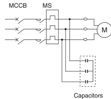
3-8 Selecting an MCCB for capacitor circuit
