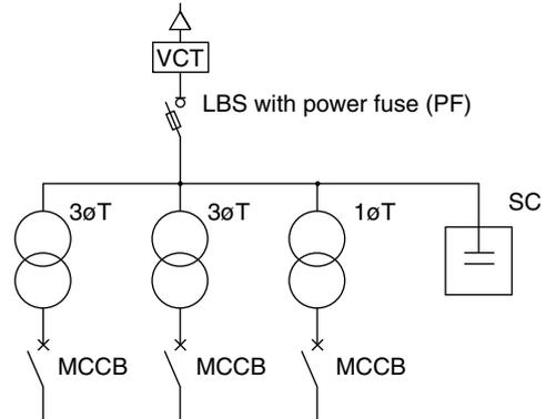
Fig. 3-8 PF high-voltage power receiving facility
