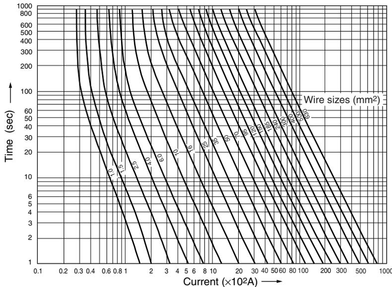
**Table 3-11a PVC wiring protected by rated breaking capacity (for short circuits)**
