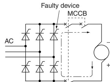
Since, in the circuit configuration shown in Fig. 3-34, the fault currents flowing through the MCCB and the devices are equal, it is necessary to meet the relation: allowable thyristor  $I^2t >$  MCCB maximum interrupting  $I^2t$  of the MCCB.
