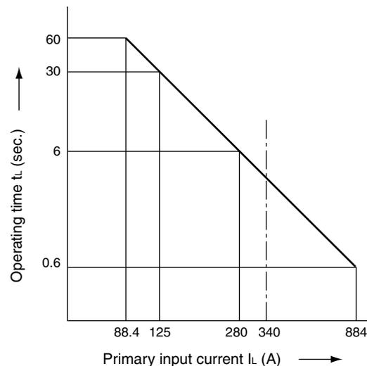
However, since the standard maximum input is prescribed for a resistance welder, even if the secondary circuit is fully shorted, the maximum short-circuit current is some 30% higher than the rated welding current (secondary current corresponding to the standard maximum input) at most. Consequently, allowance would be needed only for a value about 30% higher than the current corresponding to the standard maximum input.
