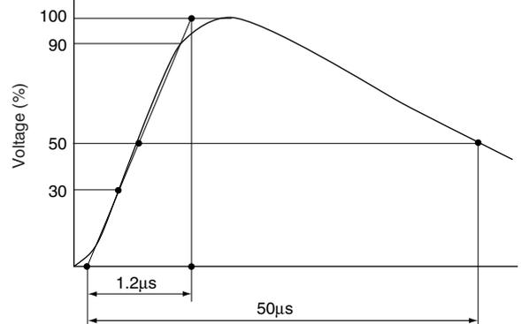
**Fig. 2-14 Evaluating MCCBs by waveform observation**
