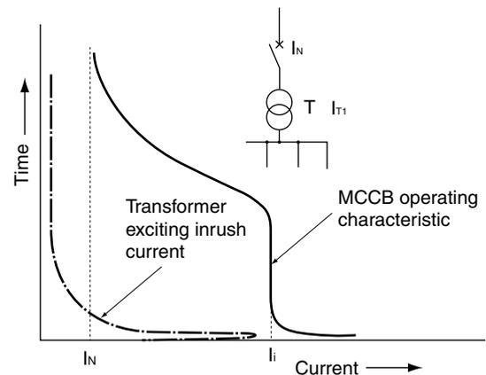
To select an MCCB for line protection, if the instantaneous trip current ( $I_i$ ) is eight times the rated MCCB current ( $I_n$ ), and the transformer exciting inrush current multiplier ( $k$ ) is 20 (typical value for 100kVA class transformers), the following relation holds:
