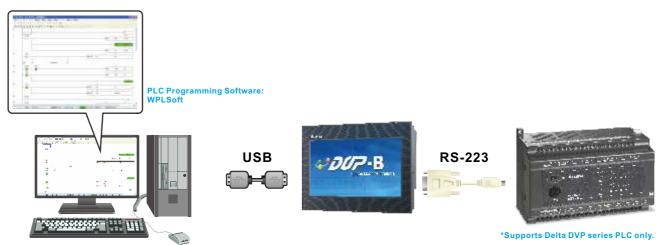
Using bypass function, enable monitoring functions and modify PLC programs directly via USB connection.
