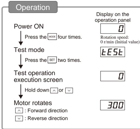
Before moving to the execution screen, if the FWD input or REV input is being ON, "Err" will be displayed.
