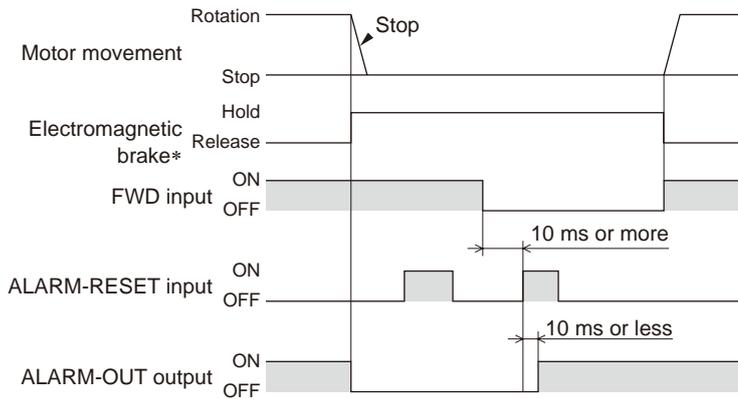
\* The electromagnetic brake will hold the shaft at the moment an alarm generates.
