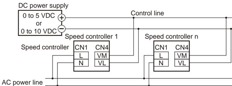
Current capacity (I) of external DC power supply when the number of speed controllers is n:
