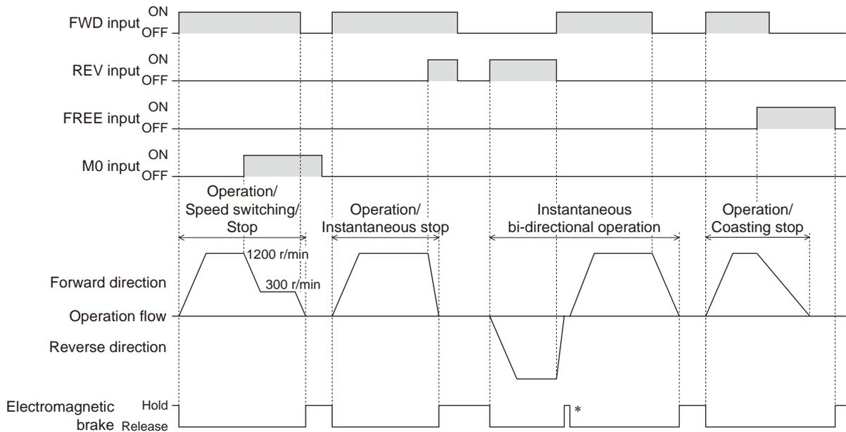
\* When the "deceleration control" parameter is set to ON, the electromagnetic brake holds (about 0.1 sec). If it is set to OFF, the electromagnetic brake will not hold.
