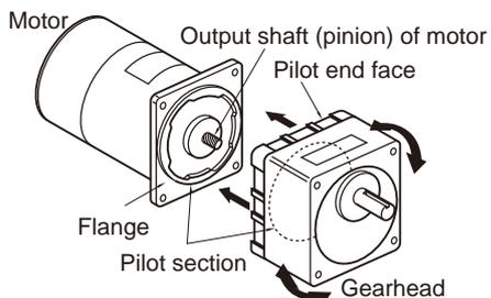
**Note** Do not forcibly assemble the motor and gearhead. Also, do not let metal objects or other foreign matters enter the gearhead. The pinion or gear of the motor output shaft may be damaged, resulting in noise or shorter service life.
