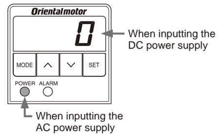
**Note** When the power is turned on, if the FWD input or REV input is being ON, the alarm code "AL 45" (prevention of operation at power-on) is displayed and the operation cannot be executed. Before supplying the power, turn both the FWD and REV inputs OFF.
