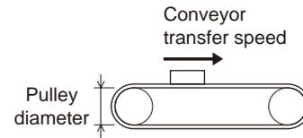
Example: The pulley diameter is 0.1 m and gear ratio of the gear head is 25
