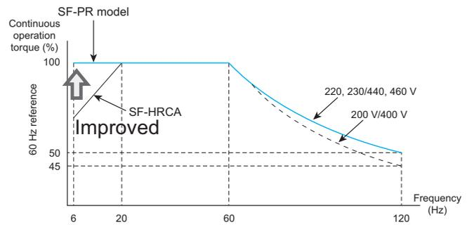
60 Hz torque reference indicates that the rated motor torque is 100% during 60 Hz operation.
