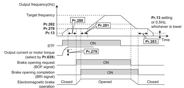
When **Pr.292** = "8" (without brake opening completion signal input)
