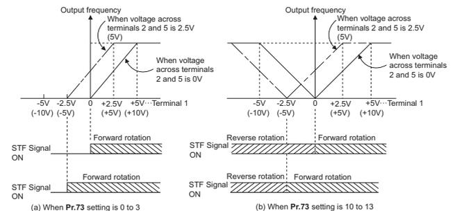
Terminal 1 (frequency setting auxiliary input) is added to terminal 2 or 4 main speed setting signal.
