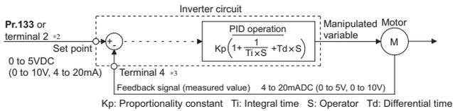
Kp: Proportionality constant Ti: Integral time S: Operator Td: Differential time
