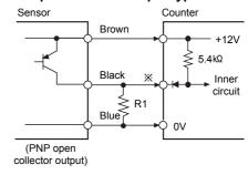
XIn case of PNP open collector output type sensor, please connect lower than 470Ω of R1 to input terminal before using.
