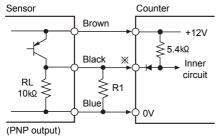
%Please set R1 value to make the composed resistance of RL + R1 as Max. 470kΩ is an impedance for short-circuit. ※CP1, CP2(INHIBIT), RESET input
