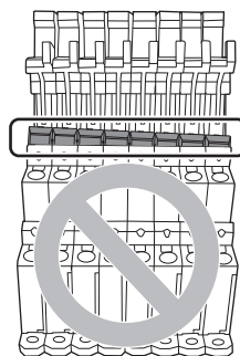
Incorrect installation Some terminals not inserted completely.
