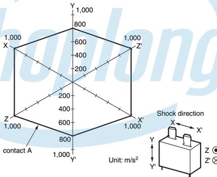
**Test Conditions:** Shock is applied in ±X, ±Y, ±Z directions three times each with and without energizing the relays to check the number of malfunctions.
