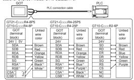
\*1 The cable for GT2103-PMBD does not have connections to the signals (RSA, RSB, CSA,CSB).
