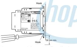
It will be easier to mount and dismount the Timer if a distance of 30 mm or more is provided between the bottom of the Timer and other equipment.
