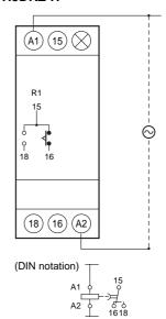
Note: The power supply terminals do not have polarity.
