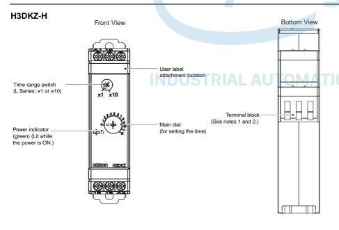
Note 1. Use solid wire (2.5 mm² max.) or ferrules with insulative sleeves to connect to the terminals.
