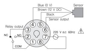
• The controller (HPA-12) for sensor has the output circuit which operates the power relay as amplifying the output of NPN type and PNP type and the power circuit for sensor. If the sensor detects an object, the relay will be operating.
