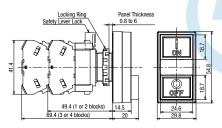
With Pilot Light Terminal screws: M3.5, integrated terminal cover Flush (top), Flush (bottom) (24V AC/DC)
