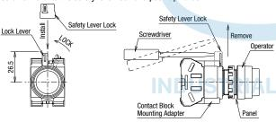
• Remove the operator from the contact block by turning the locking lever in the direction of the arrow shown below. Then the operator can be pulled out.
