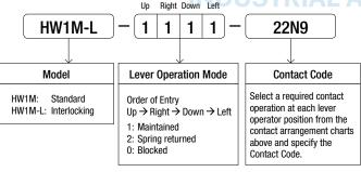
The lever operator of the interlocking type HW1M-L is locked only in the center position.
