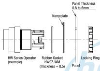
Mounting panel thickness is reduced by 1.5 mm when using a nameplate.
