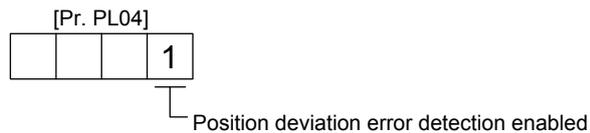
When you compare the model feedback position ( 1 )) and the feedback position ( 2 )) in figure 15.1, if the deviation is more than the value of [Pr. PL05 Position deviation error detection level] ( 1 (0.01 rev) to 1000 (10 rev)), [AL. 42.1 Servo control error by position deviation] will occur and the linear servo motor will stop. The initial value of this detection level is 0.09 rev. Replace the set value as required.
