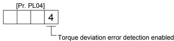
When you compare the command torque ( 5)) and the feedback torque ( 6)) in figure 15.1, if the deviation is more than the value of [Pr. PL07 Torque/thrust deviation error detection level] (1% to 1000%), [AL. 42.3 Servo control error by torque/thrust deviation] will occur and the linear servo motor will stop. The initial value of this detection level is 100%. Replace the set value as required.
