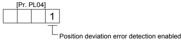
When you compare the model feedback position ( 1)) and the feedback position ( 2)) in figure 14.1, if the deviation is more than the value of [Pr. PL05 Position deviation error detection level] (1 mm to 1000 mm), [AL. 42.1 Servo control error by position deviation] will occur and the linear servo motor will stop. The initial value of this detection level is 50 mm. Replace the set value as required.
