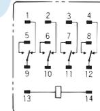
(The coil has no polarity.)
