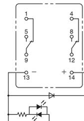
**Note:** For the DC models, check the coil polarity when wiring and wire all connections correctly.
