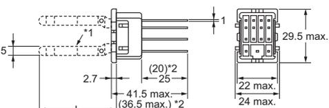
\*1. PY14QN-Y□ and PY14QN2-Y□ include the portion indicated by broken line.
