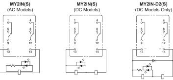
Note: For the DC models, check the coil polarity when wiring and wire all connections correctly.
