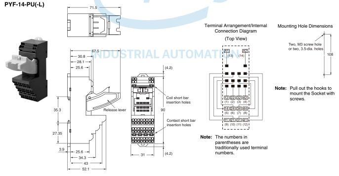
\*The PYF-14-PU-L Sockets do not have release levers.
