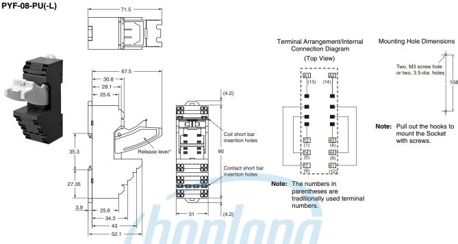
\* The PYF-08-PU-L Sockets do not have release levers.
