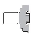
Use two M3 screws to mount the case-surface mounting (MY□F) and tighten them securely. (Appropriate tightening torque: 0.98 N·m)
