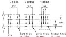
The dimensional tolerance is ±0.1. Note: 1. Refer to the terminal arrangement and internal connections diagrams for the MY2, MY3, MY4, and MY4Z.
