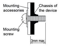
Fig. 4 Mounting Screw
