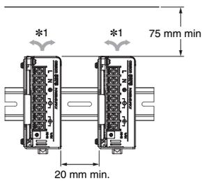
The above figure shows a model with the terminal block facing forward.
