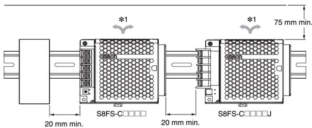
To mount the Power Supply to a DIN Rail, hook portion (A) of the Power Supply onto the DIN Rail and press the Power Supply in direction (B) until you hear it lock into place. Make sure that the catch on the Mounting Bracket is engaged with the DIN Rail.
