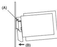
To dismount the Power Supply, pull down portion (C) with a flat-blade screwdriver and pull out the Power Supply.
