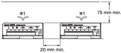
The above figure shows a model with the terminal block facing upward.
