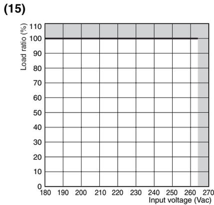
**Note:** The internal parts may occasionally deteriorate or be damaged. Use the standard mounting method only. Do not use the Power Supply in the area outside the derating curve.
