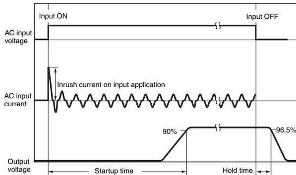
**Note:** Twice the normal input current will flow for a redundant system. Sufficiently check the fusing characteristics of fuses and the operating characteristics of breakers and select fuses and breakers so that external fuses will not burn out or breakers will not operate due to inrush current.
