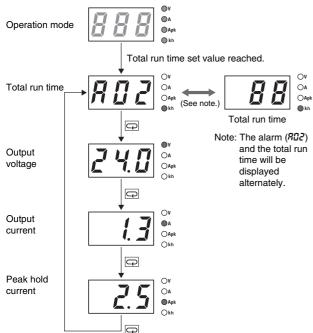
The accumulated value of the operating time of the Power Supply is displayed as the total run time.  $\it I$  (kh) will be displayed initially after purchase and then the display will advance in *I*-kh steps as the operating time accumulates. When the total run time reaches the alarm set value, the alarm (RD2) and the total run time will be displayed alternately and a transistor (total run time output terminal (kh)) will output the status externally.
