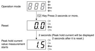
Note: The peak hold current value is not reset in the setting mode.
