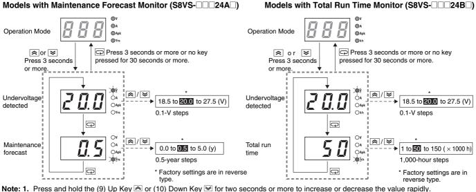
2. The S8VS-06024 is not provided with the setting mode and its parameters are fixed at the shipment setting.
