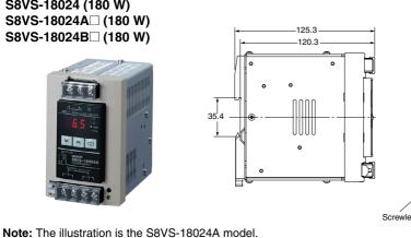
Seven, M4 terminal screws with square washers +10+ 8.8.8. 888 115 00 4.5 -75 Rail stopper (Sliding: 15 max.) Screwless block (2.5-mm pitches)
