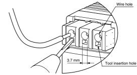
• Use the following material for the wires to be connected to the S8VS to prevent smoking or ignition caused by abnormal loads.
