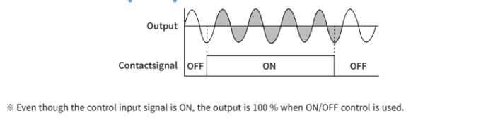
• Even though the control input signal is ON, the output is 100% when ON/OFF control is used.
