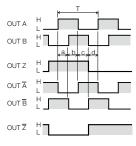
a, b, c, d = 1/4T±1/8T Note: Clockwise rotation when the main body is the axle side is the normal rotation.
