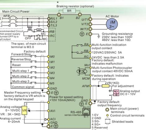
NOTE: Do not plug a Modem or telephone line to the RS-485 communication port, permanent damage may result. Terminal 1& 2 are the power sources for the optional copy keypad and should not be used while using RS-485 communication.
